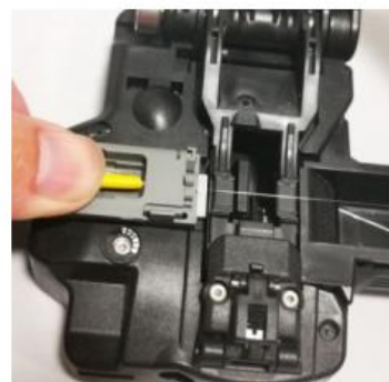
8. Using cleaver cut the bare fiber
