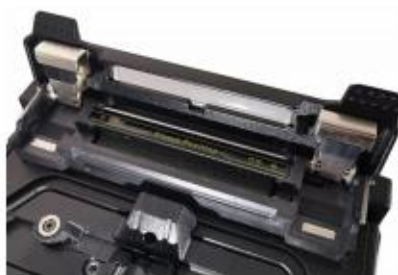
Inductive heater, without fiber not heating
