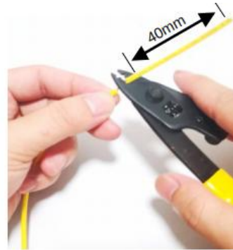
2. Strip off the jacket at a reserved place of about 40mm
