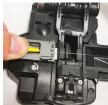
8. Using cleaver cut the bare fiber
