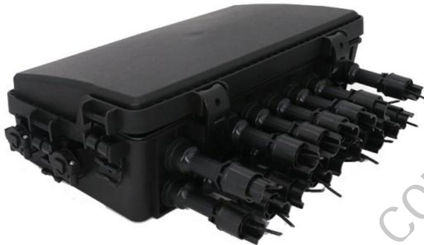
MT-1526 fiber optic box are specially designed to protect joints of optic cable. Excessive fibers can be stored in storage baskets behind the splice trays. The optical fibers are fusion on sides of the tray. Adopt modified PP material, with anti-UV, anti-aging and corrosion resistance material. Good quality and long service life. It is reusable.
